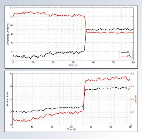
Graphs showing the capability of the exhaust system to monitor emissions (Upper) and the effect of varying throttle position (Lower).
