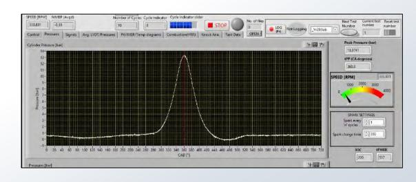
Streamlined graphical user interface allowing for complete control of spark and injection timing, and throttle position.
