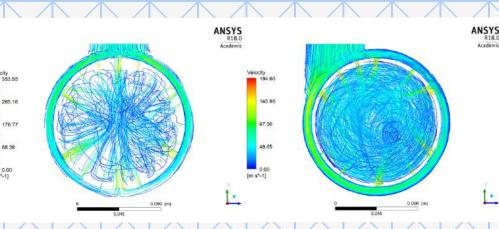
Left Image: The holes (size and location) drilled into the liner were designed in an iterative manner to give the required airflow distribution of 50-20-30% into the primary, secondary and dilution zones of the combustion chamber.
