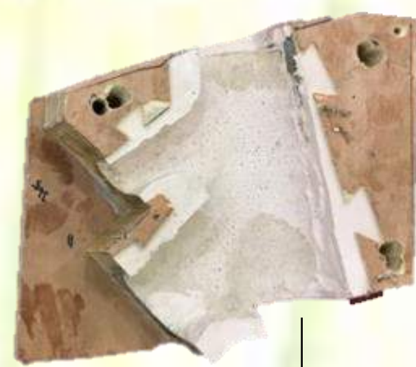
Plywood (negative mould) By CNC machine
