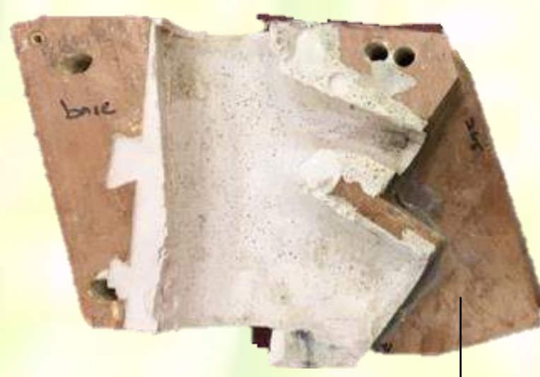
Plywood (negative mould) By CNC machine
